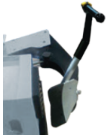
BEAD BREAKER CONTROL BY LEVER
