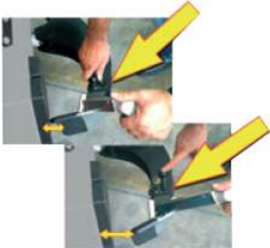
BEAD BREAKER ADAPTOR WITH TILTING ADJUSTABLE
