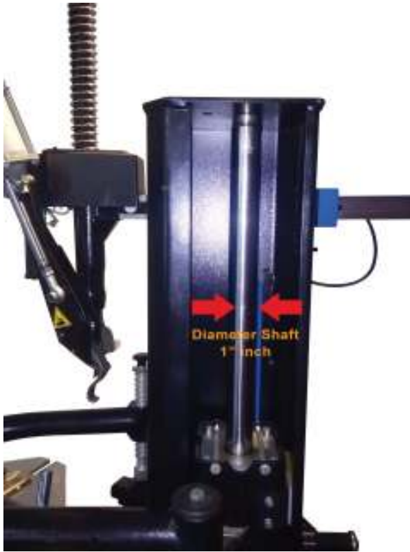
Piston Shaft diameter 1"
